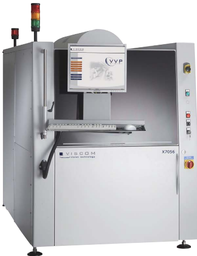
Viscom's X7056 combined AOI/AXI machine performs simultaneous optical and 3-D x-ray inspection of PCBs with dense, complex component packages like ball-grid arrays.
